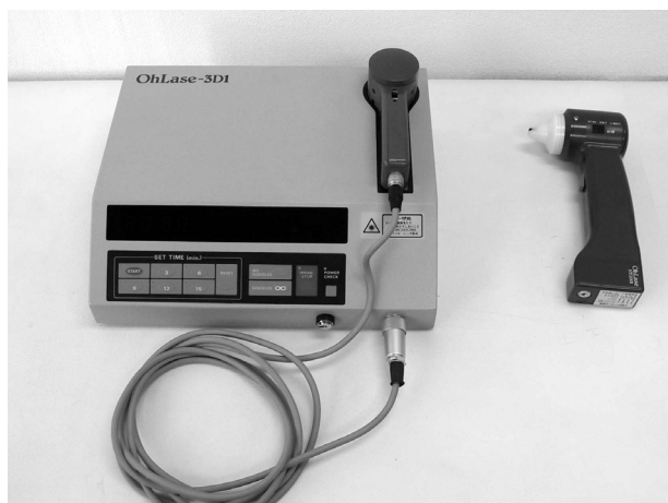
Fig 1: The OhLase-3D1. (Left) Console type, consisting of a control console linked to the hand-held probe by a control cable. (Right) OhLase-3D1-HT portable, rechargeable battery-powered version, same parameters as the console type.
